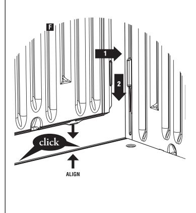
Install Wall Connector (Q) 5 places, connecting Left Back and Right Back Panels (D and F). Position connectors in slots and slide down to snap in place.
